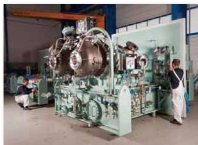
Cryostar's 4 Stage Gas Compressor for LNG Carriers with DFDE Engines
