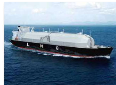
Continuous Tank Cover Spherical Tank LNG Carrier, “SAYAENDO” (Photo courtesy of the Nagasaki Shipyard and Machinery Works of Mitsubishi Heavy Industries, Ltd.)
